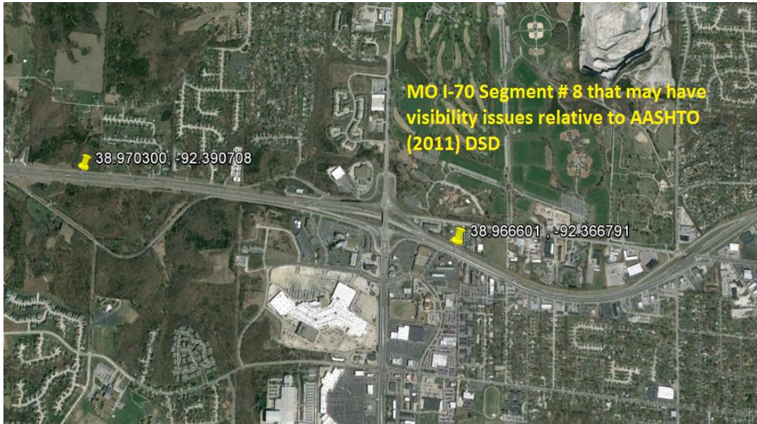
Figure 5.15: MO I-70 segment 8 with potential visibility issues
